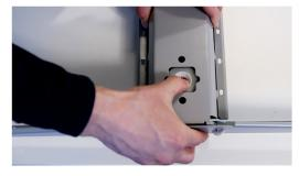
Easily install the crossbeam to the worksurface with the cantilevers. The cantilevers snap in place and then the cantilevers and the crossbeam need to be screwed to the worksurface.
